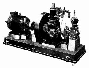
In the absence of one of these stand-by sets, the air reservoirs are usually charged (for the initial start after installation) by means of a bottle of highly compressed air which is readily obtainable in most districts. Failing this, a hand pump is used, but this method of initial charging is both long and laborious.
